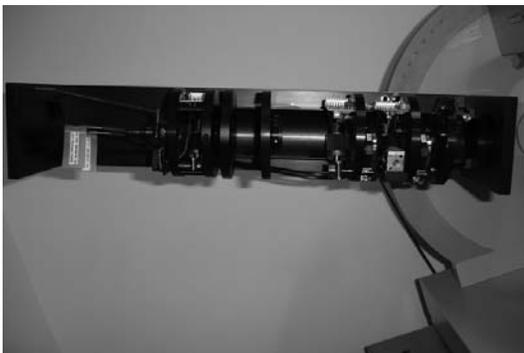
(a) The input box of the ellipsometer..
