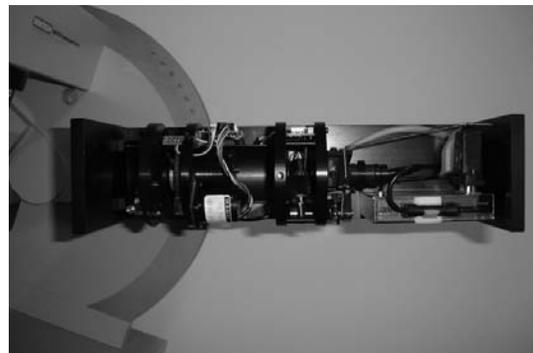
(b) The output box of the ellipsometer.
