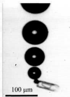
Figure 2.16: CO 2 bubbles nucleating from champagne at the bottom of a glass. Here, gas pockets entrapped inside cellulose particles serve as nucleation sites. The images, taken with a high speed video microscope, were kindly provided by G. Liger-Belair [40].
