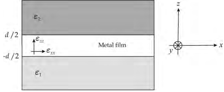
Figure 30.2. Schematic geometry of an anisotropic metal film sandwiched between isotropic dielectrics.
