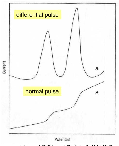
mixture of Cd<sup>2+</sup> and Pb<sup>2+</sup> in 0.1M HNO<sub>3</sub>.
