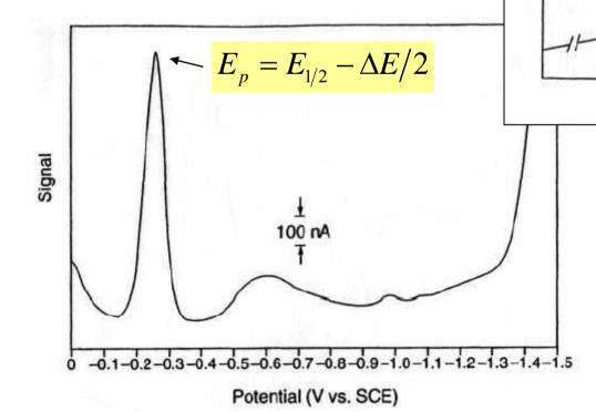
$$i_{p}(t) = \frac{nFAD_{o}C_{o}(b)}{\sqrt{\pi D_{o}t_{m}}} \left(\frac{1-\sigma}{1+\sigma}\right)$$
