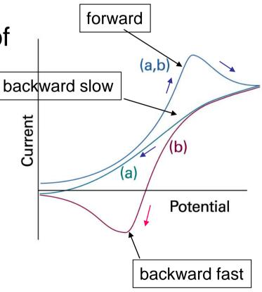
In the case of adsorption process on the electrode, the separation between the peaks will be smaller and current will be proportional to the adsorption
