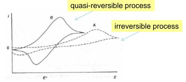
$$E_{p} = E^{\circ} - \frac{RT}{\alpha n_{a}F} \left[ 0.78 - \ln \frac{\mathbf{k}^{\circ}}{\mathbf{D}^{1/2}} + \ln \left( \frac{\alpha n_{a}Fv}{RT} \right)^{1/2} \right]$$
