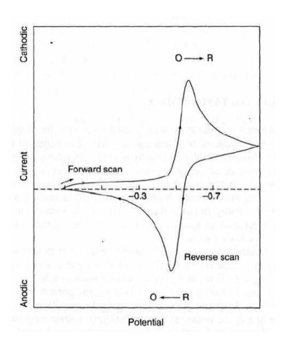
For irreversible processes (where electron transfer is a limiting factor) peak potential will depend on the scan rate
