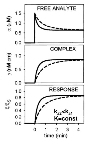
$$\frac{d\gamma}{dt} = k_a \left(\alpha_0 - \frac{S}{V}\gamma\right) (\beta - \gamma) - k_d \gamma$$
