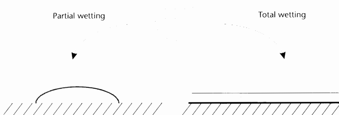
Figure 2.7 Partial wetting and total wetting.
