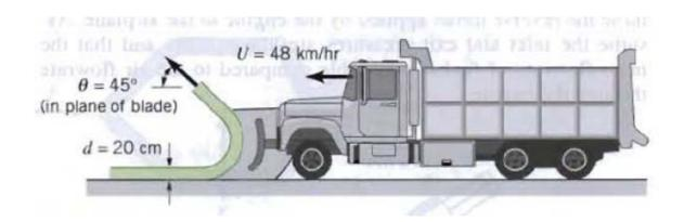
**Solution**. From the Reynolds transport theorem in the coordinates of the moving truck:
