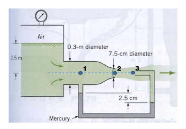
**Solution.** First we apply the Bernoulli equation between the points 1 and 3:
