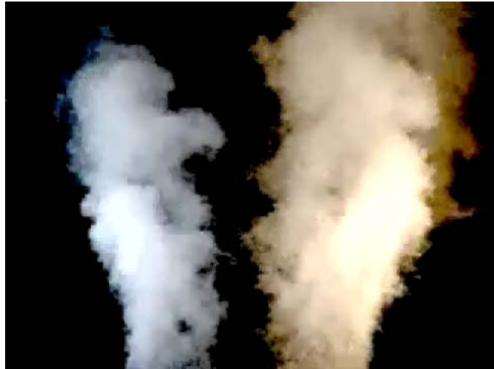
The flow generated by an airplane is made visible by flying a model Airbus airplane through two plumes of smoke. The complex, unsteady, three-dimensional swirling motion generated at the wing tips (called trailing vortices) is clearly visible
